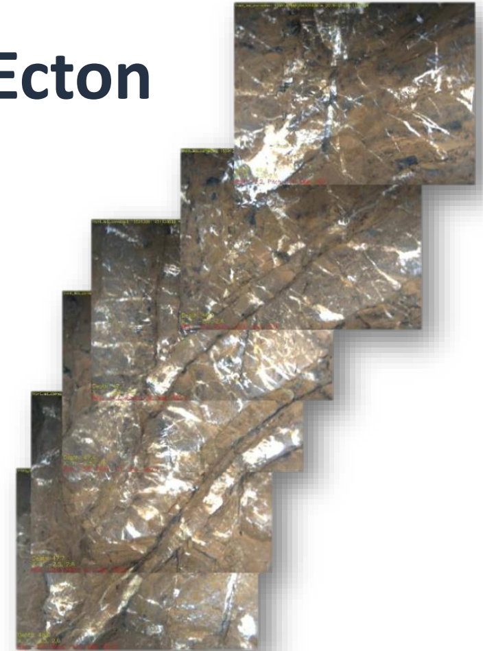
Syncline with calcitized tension cracks, winding shaft (-46-48 m)
